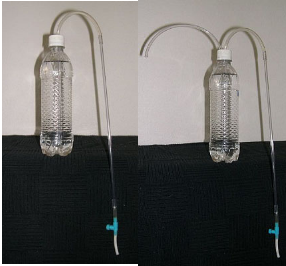
The assembled kalk dripper. Note the siphon tube installed in the picture on the right.
